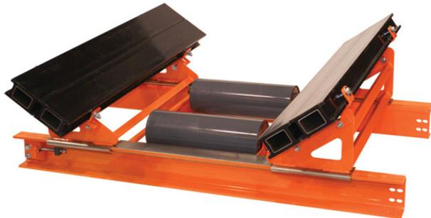
The **Martin® Modular Slider Cradle** utilizes low friction UHMW bars to support the belt at the outside of the load-carrying area. This stabilizes the belt line, eliminating the sag and bounce that spill material, and reducing the risk of catching lumps that can abrade the belt surface.
